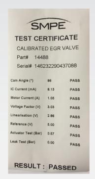
All components are reassembled before the unit is calibrated and tested. This procedure accurately calibrates the electronic feedback of the valve. The coolant section is then pressure tested to detect any leaks. The final test is to flow gasses through the unit at various pressures and rates to ensure the correct electronic signal is produced.
