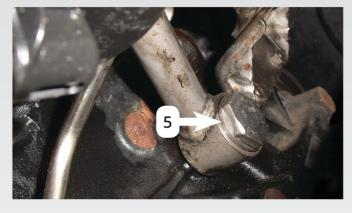
Remove bolts and banjo bolt then detach support for turbocharger with oil supply line (5)
