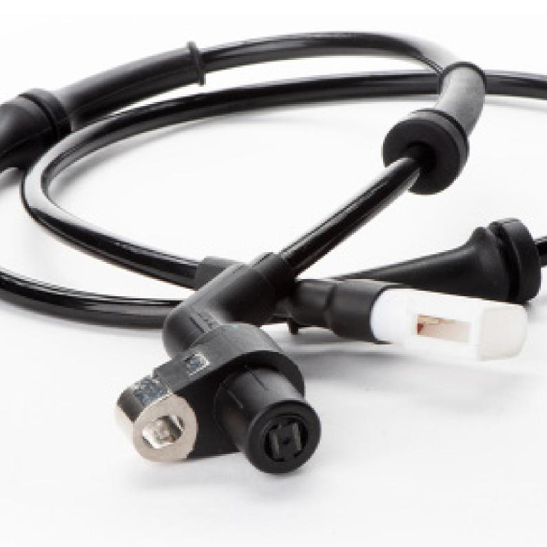
Please note the different types of ABS/wheel speed sensor, there are generally four types. An initial distinction can be made between active and passive ABS sensors. Active ABS sensors can be recognised when they are new by their being
